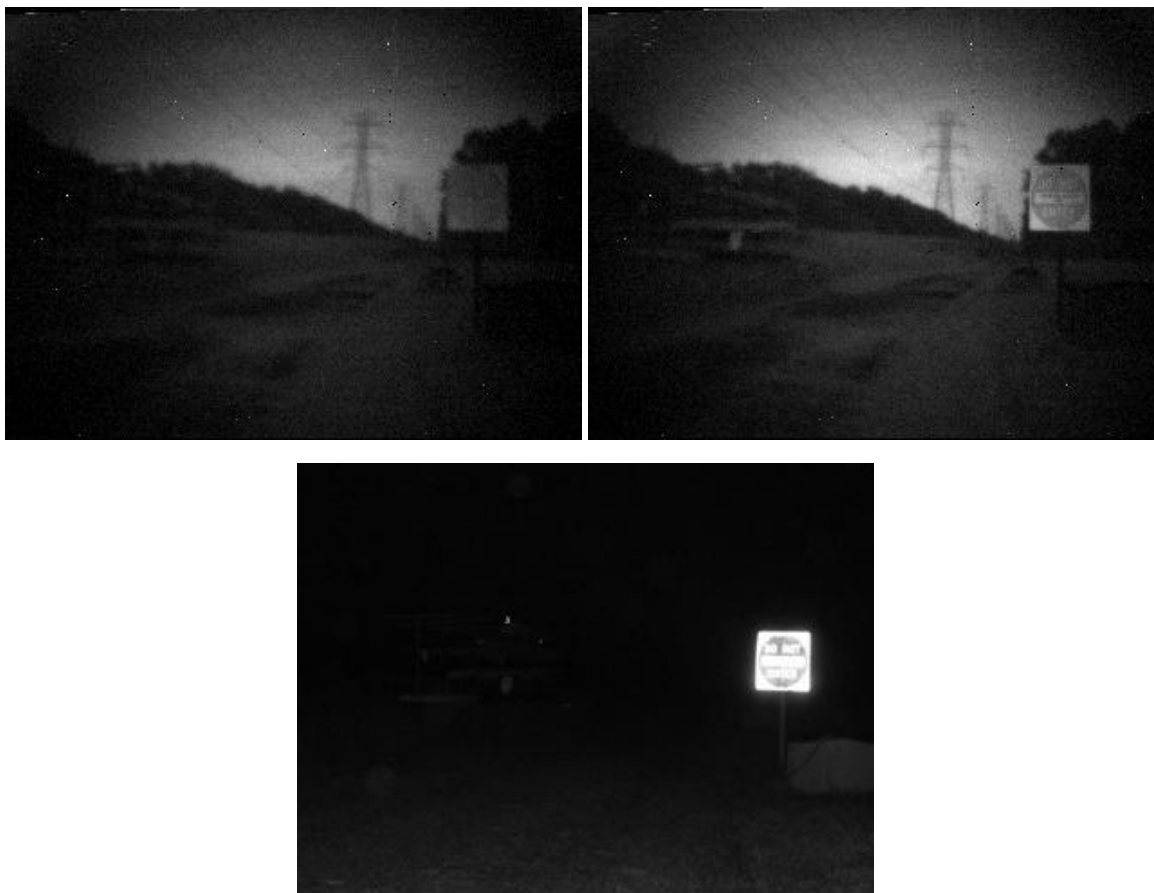
Figure 7. Pictures taken at night along a dark road. Top left taken with SWIR InGaAs camera. Top right taken with Visible InGaAs™ camera (SWIR + visible). Bottom taken with visible camera.
